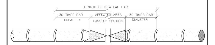
IF REBAR HAS LOST MORE THAN 25% OF ORIGINAL CROSS SECTION, PROVIDE NEW LAP BAR AS SHOWN
