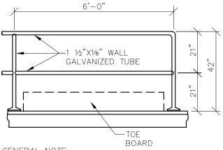
INSTALL A TOE BOARD PER MDCIS GENERAL INDUSTRY SAFETY STANDARD, PART 2. WHERE PEOPLE PASS UNDERNEATH, THERE IS MOVING EQUIPMENT, OR THERE ARE EQUIPMENT OR TOOLS THAT COULD FALL.
