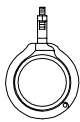
ADJ. SWIVEL PIPE RING SPLIT RING TYPE OR SOLID RING TYPE TYPE-6
